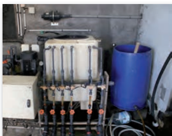
Station de fertigation type Heliotec ®.
